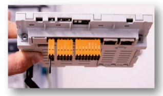
Figure 6.2.2.b: GEN24 Pilot connection area
